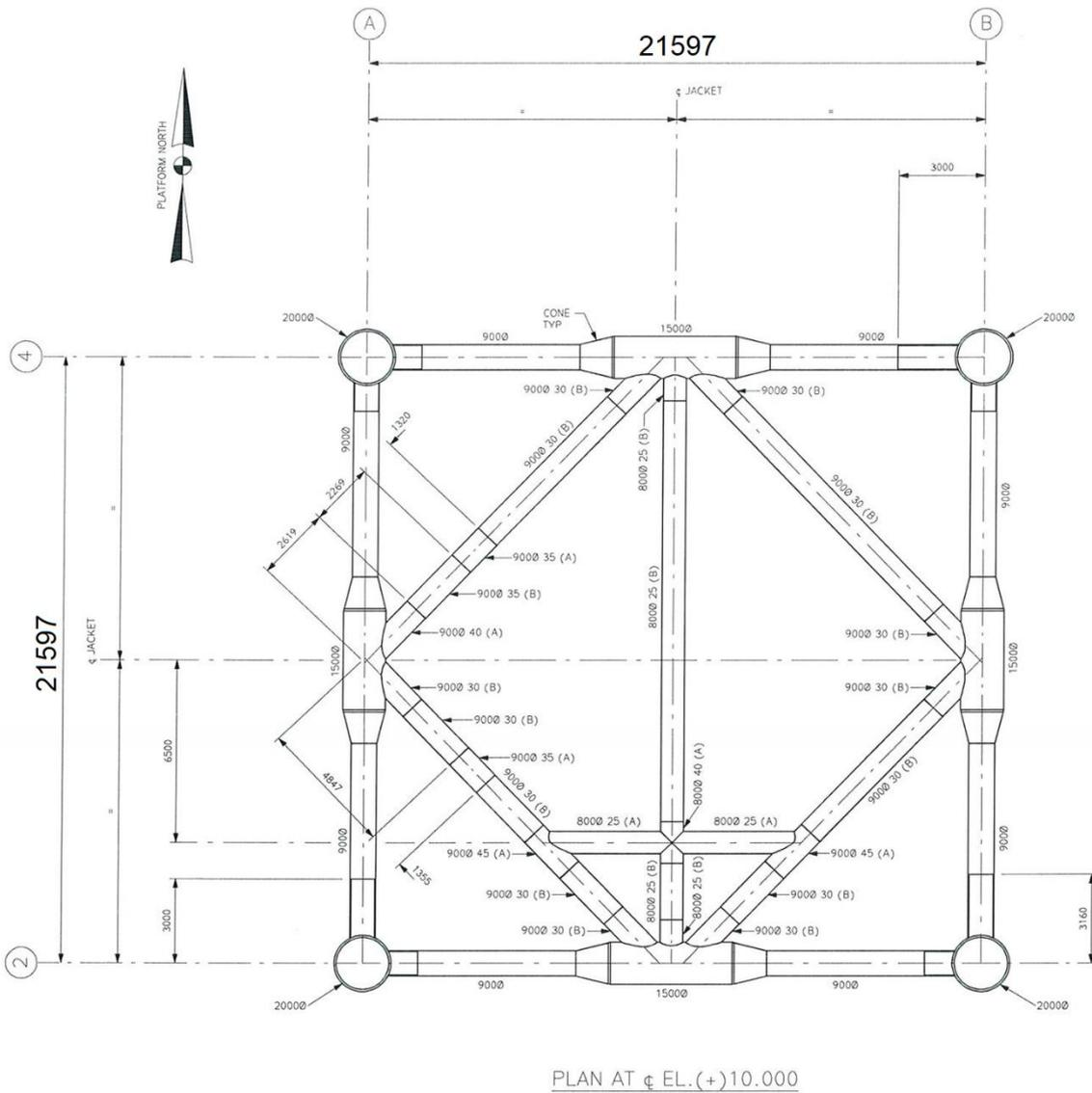
**Figure 3.2.5: Solan jacket bracing plan at EL. +10.000**
