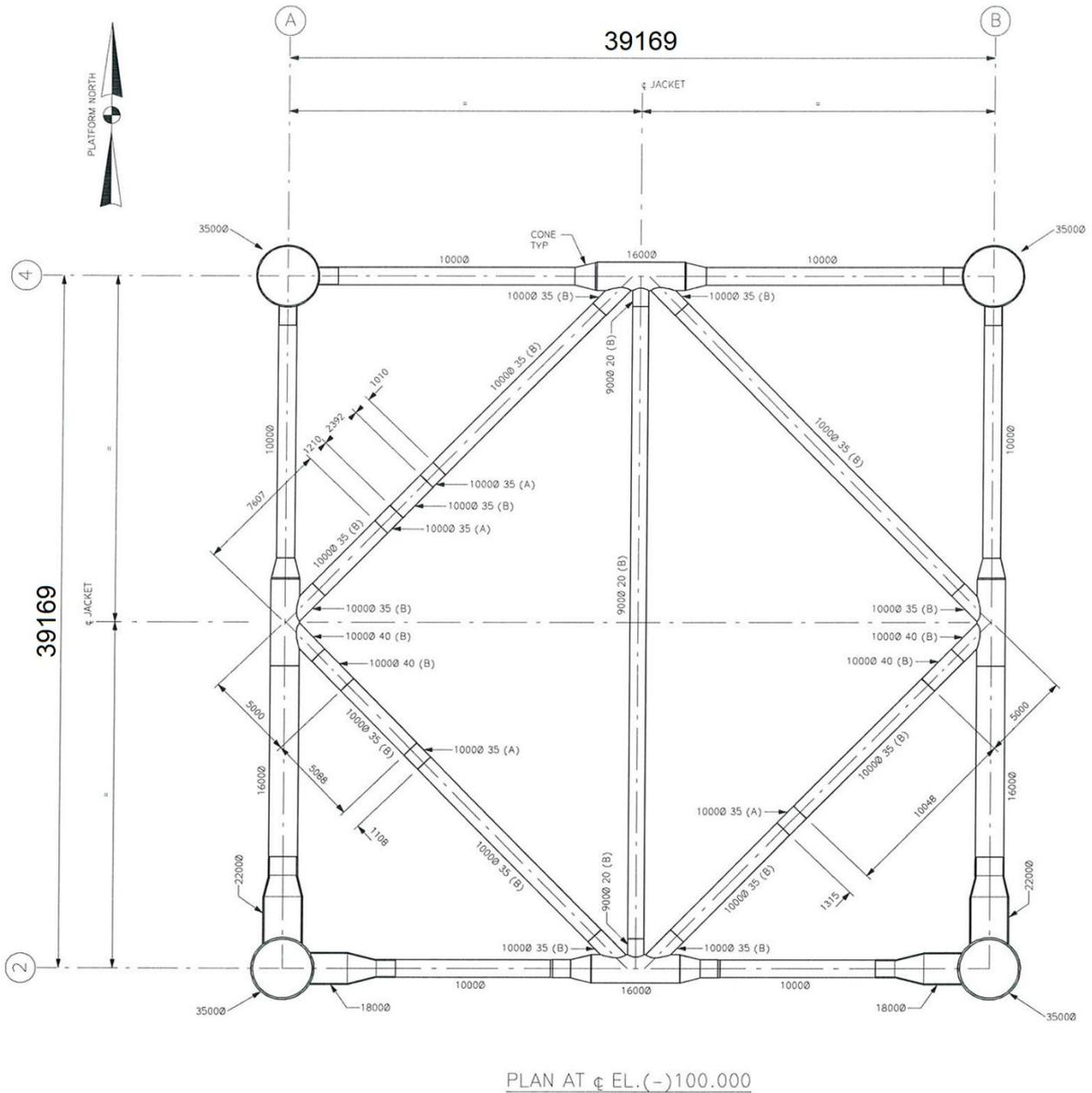
**Figure 3.2.9: Solan jacket bracing plan at EL. -100.000**
