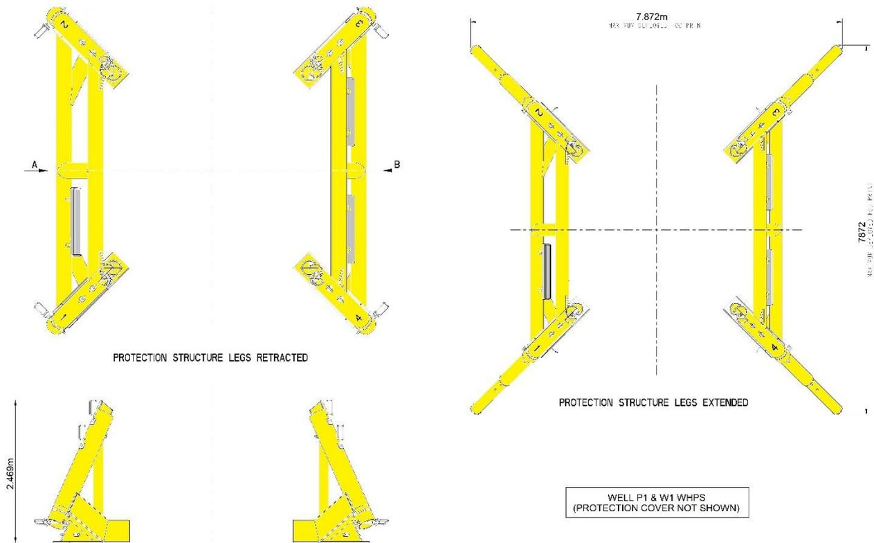
**Figure 2.2.4: Plan view on WHPS for well P1 & W1 (protection cover not shown)**
