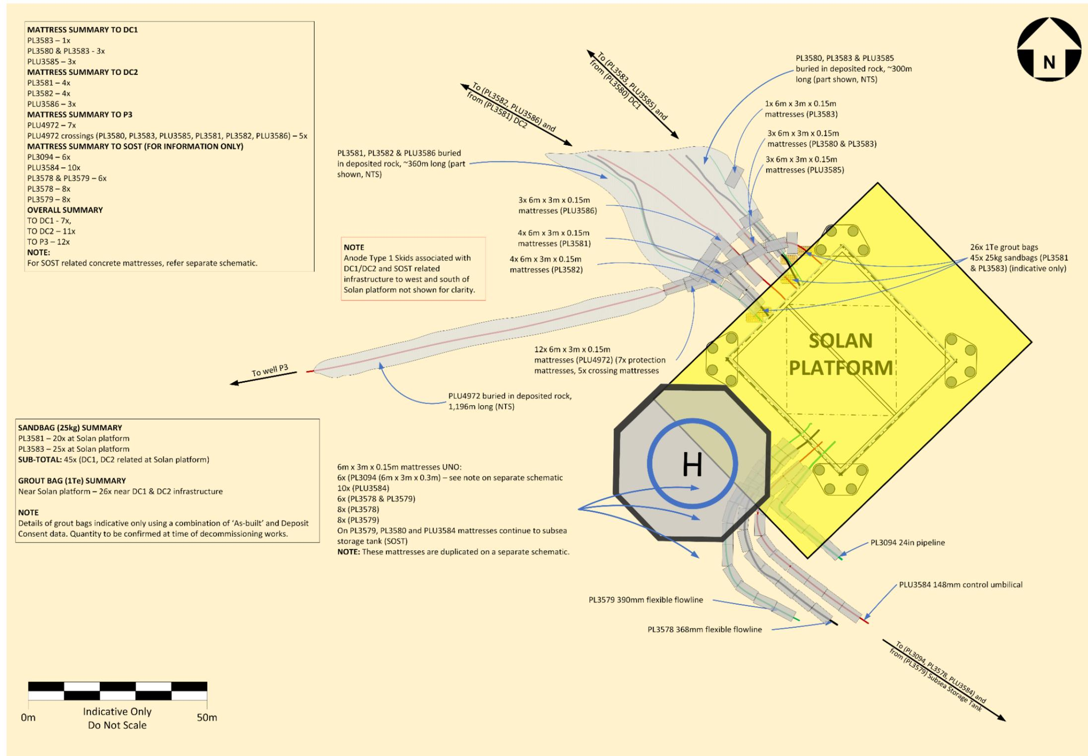
Figure 6.6.2: Solan platform approach schematic
