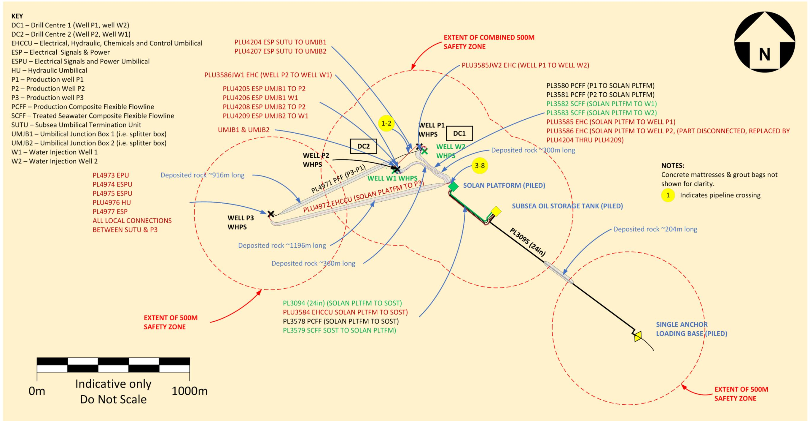
Figure 6.6.1: Solan field infrastructure overview schematic
