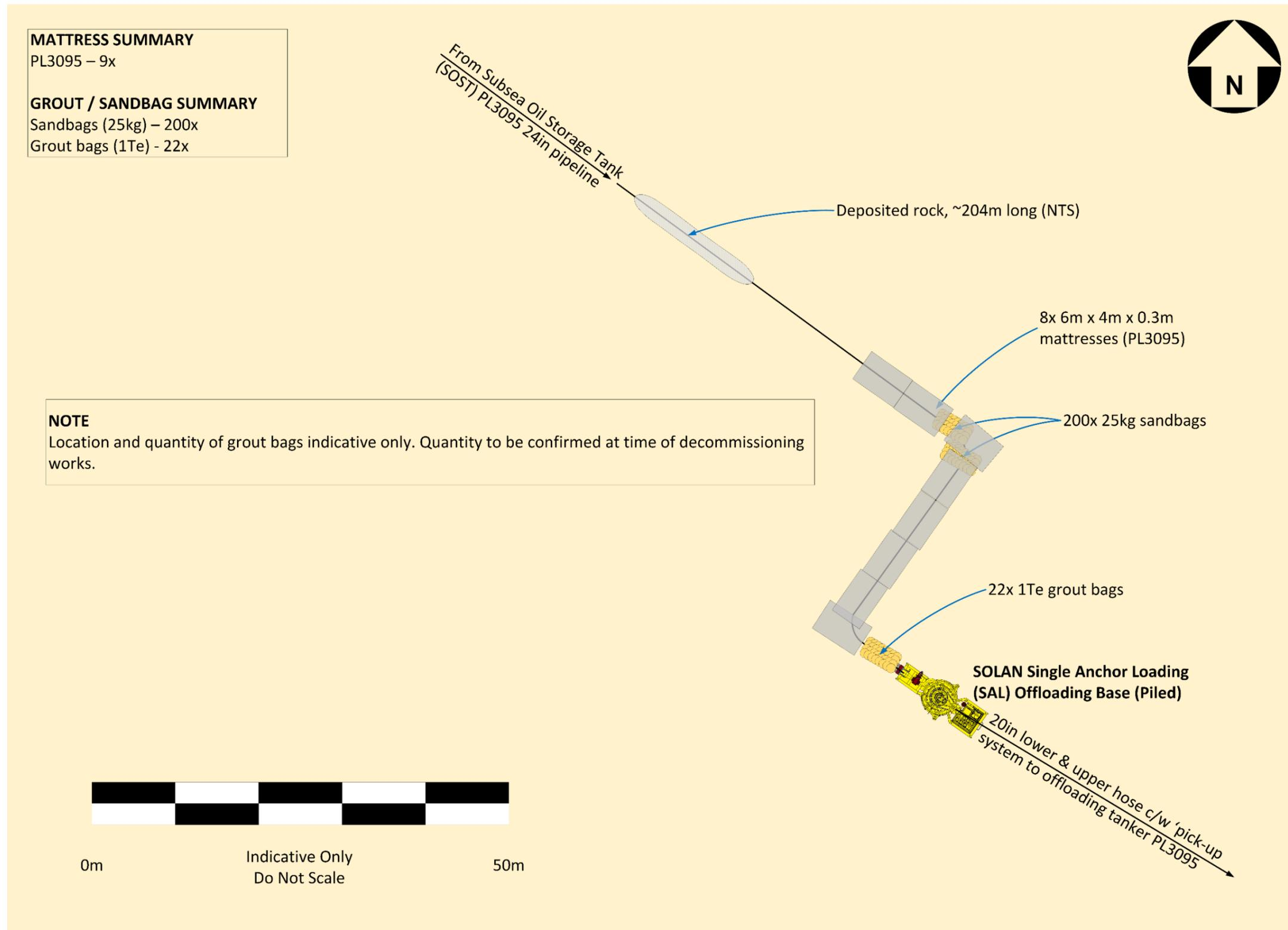
Figure 6.6.4: SAL approach schematic
