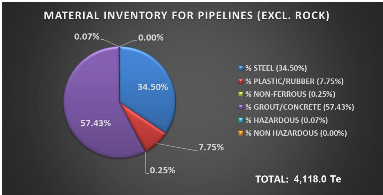
Figure 2.7.2: Material inventory for Solan pipelines<sup>3,4</sup>
