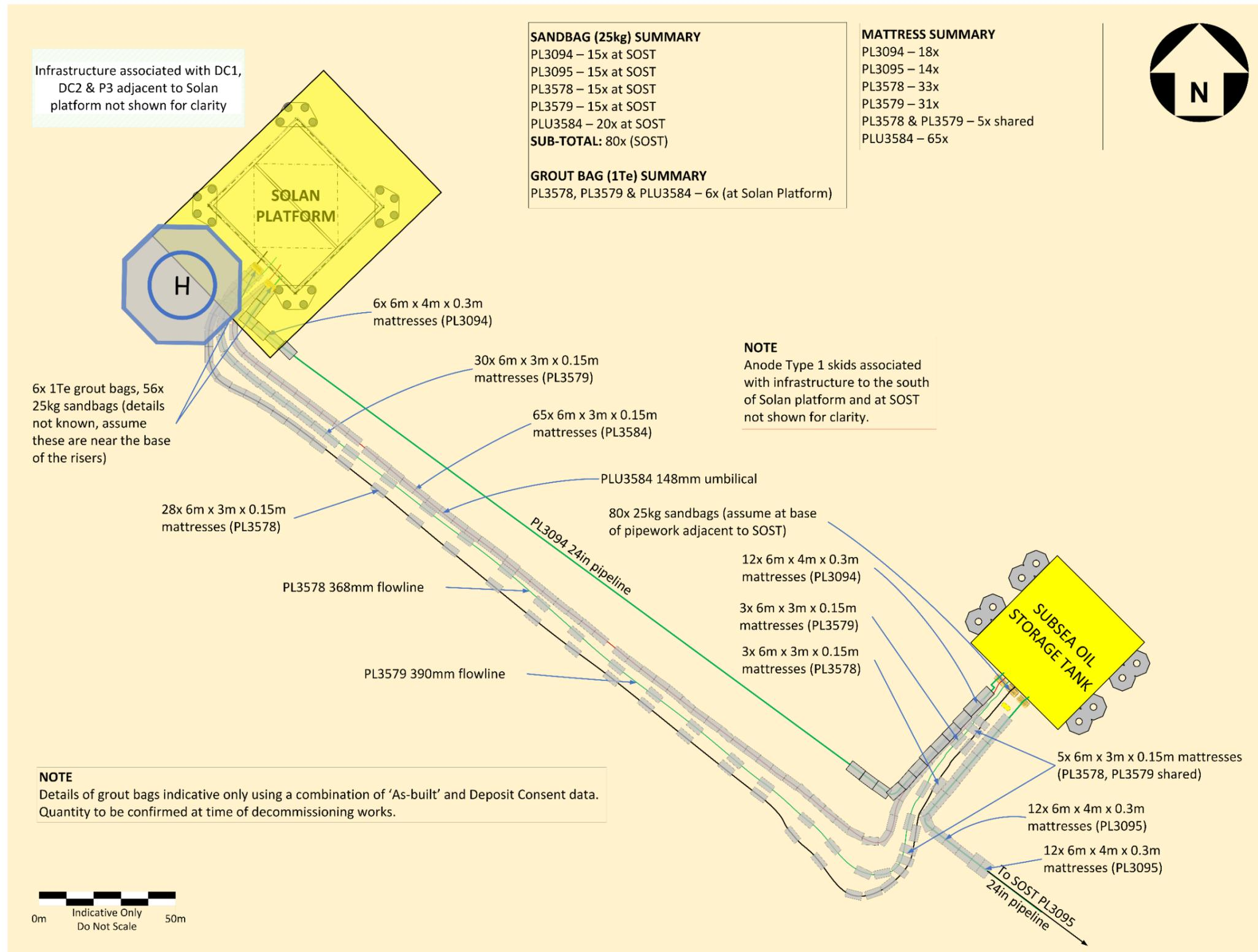
Figure 6.6.3: Solan platform and SOST infrastructure schematic
