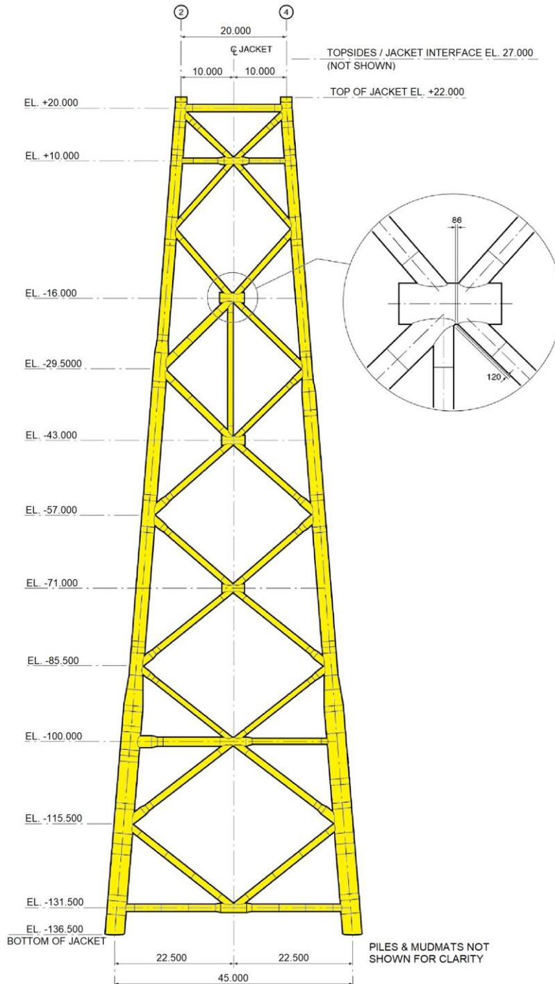
**Figure 3.2.3: Solan jacket elevation on row 'A' (rows 'B', '2' & '4' similar)**
