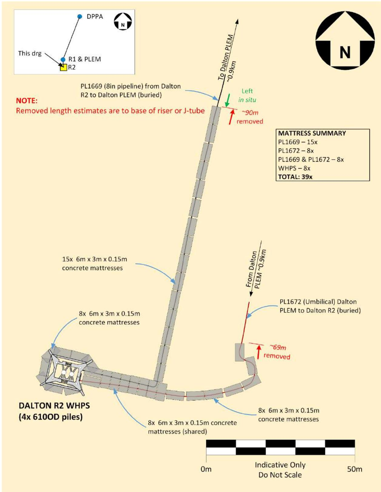
Figure 3.2.2 Dalton Well R2 approach schematic
