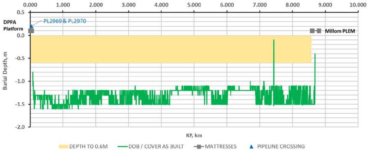
**Electric & fibre-optic cable 113mm nom dia. DPPA to Millom West (as-built)**
