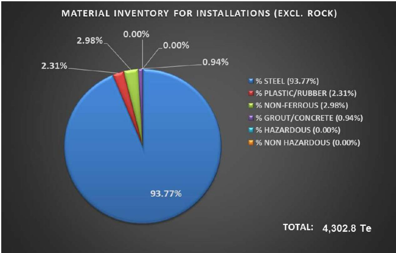
Figure 3.9.2 Pie-chart of material inventory for Calder, Dalton & Millom installations<sup>2</sup>
