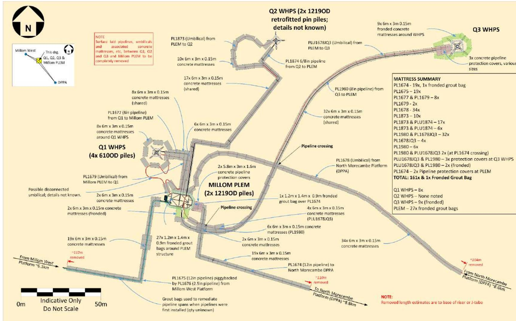
Figure 3.2.3 Millom PLEM, Well Q1 & Q3 approach schematic
