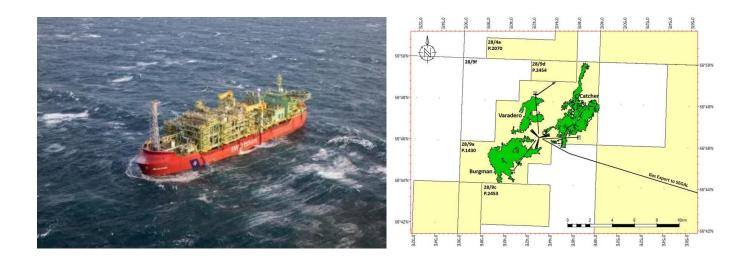
The *BW Catcher* is a Floating Production, Storage and Offloading facility (FPSO) that is located 173 kilometres to the SE of Aberdeen. The *BW Catcher* currently produces from three fields (Catcher, Varadero and Burgman). These three fields have 15 producers and four injectors. The *BW Catcher* was installed in 2017. First oil was late in that year. A programme of development drilling is planned by operator.
