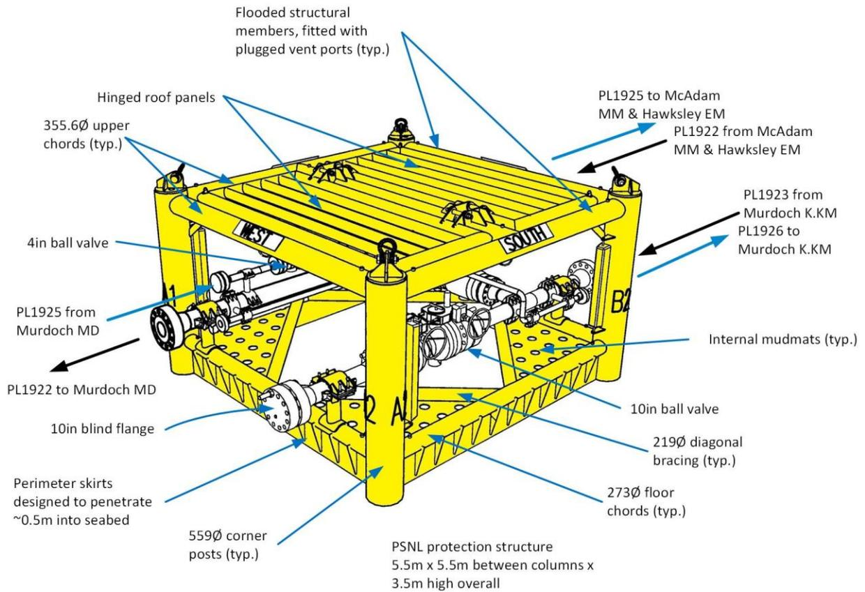
Figure 2.3.6: Perspective of the PSNL protection structure
