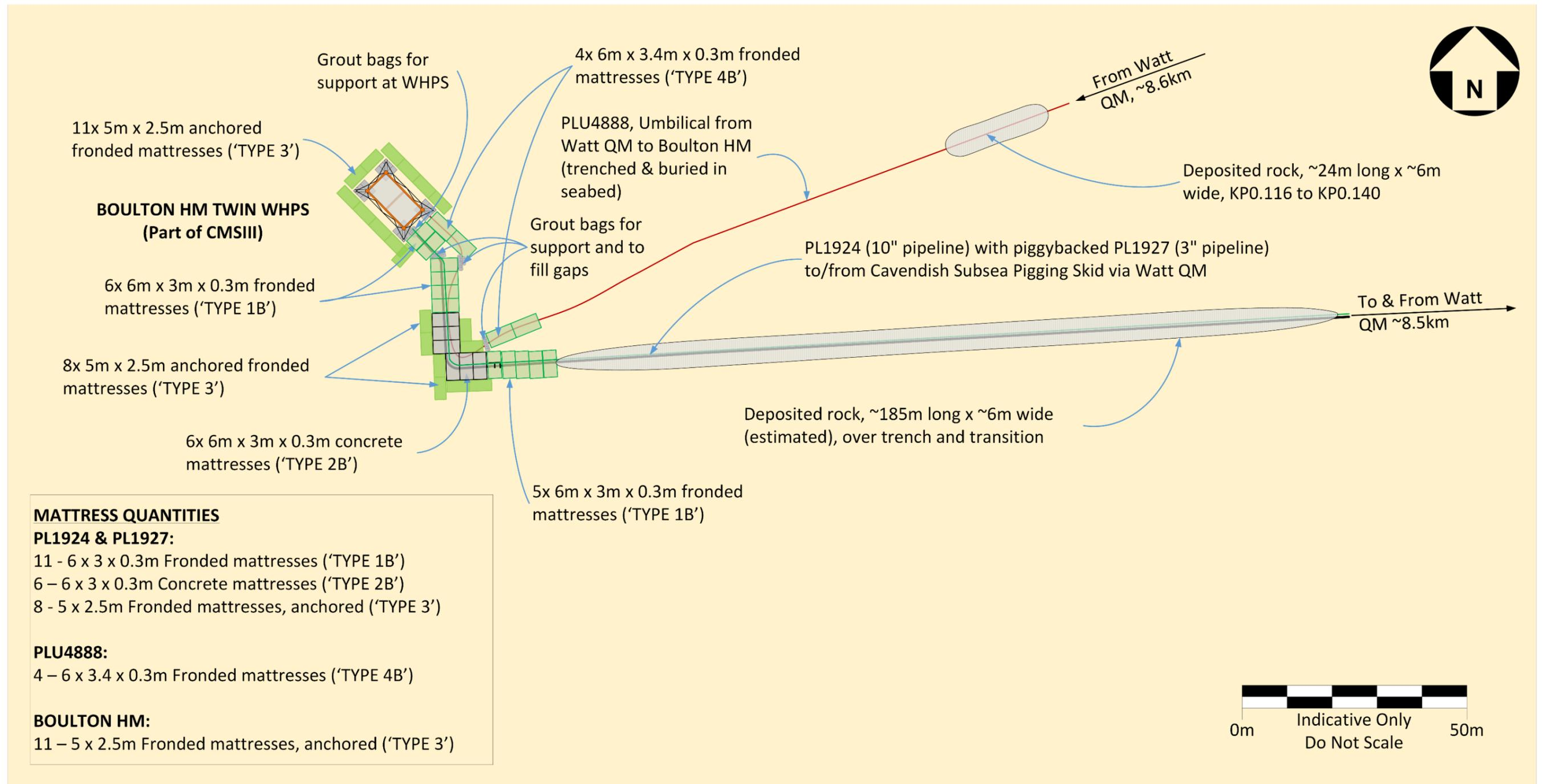
Figure A1.3.1: Schematic of pipelines near Boulton HM
