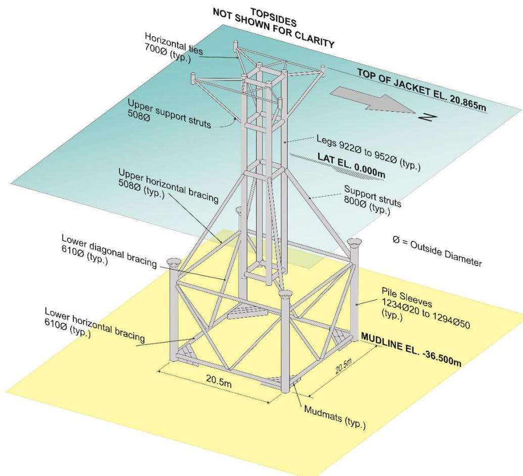
Figure 3.2.1: Boulton BM jacket 3D view
