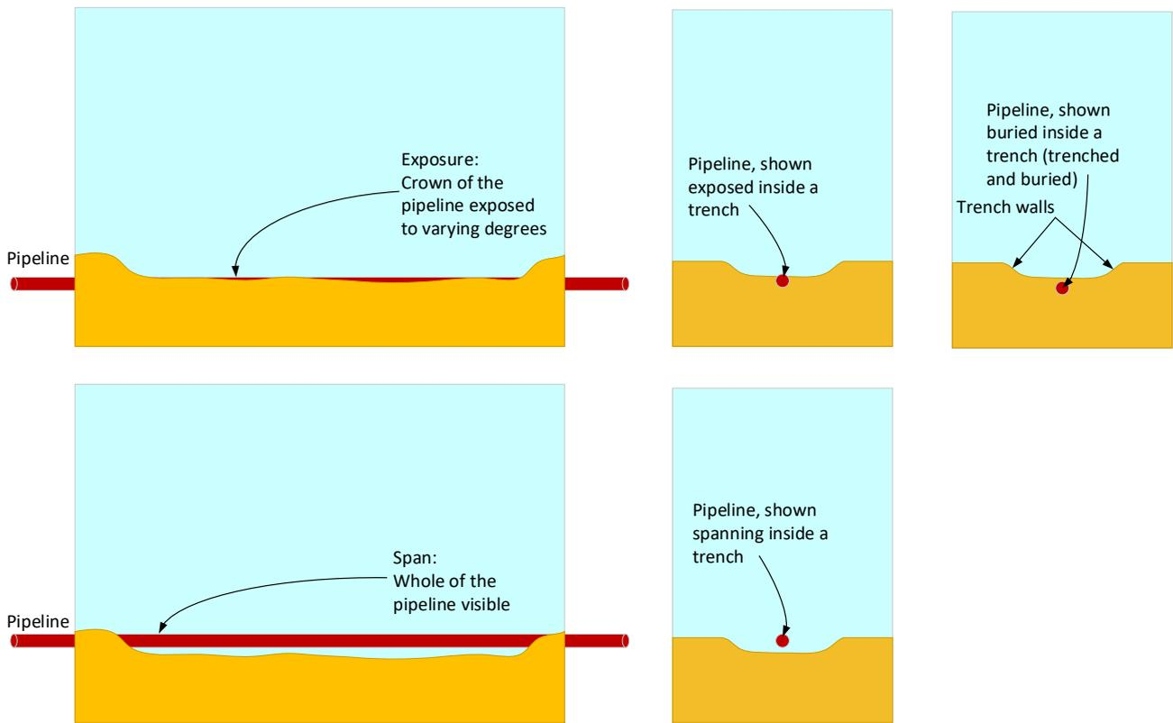
Figure 1.1.1: The difference between pipeline burial, exposures, and spans<sup>1</sup>
