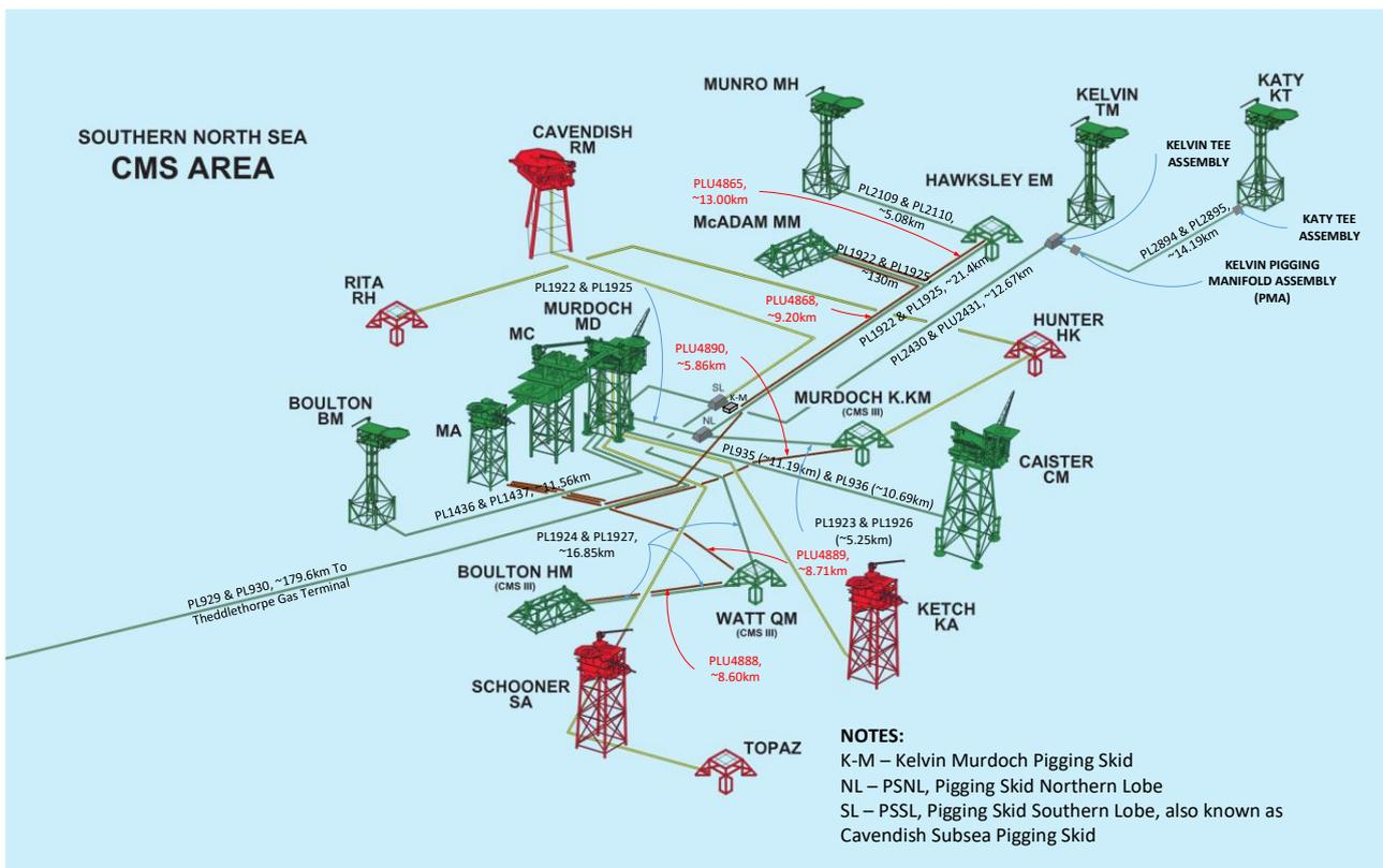
Figure 1.3.1: Murdoch and CMS area installations and pipelines
