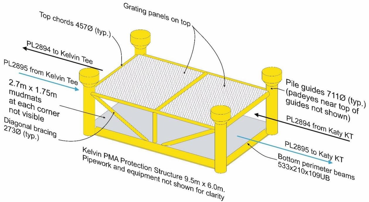
**Figure 2.3.3: Perspective of the Kelvin PMA protection structure**
