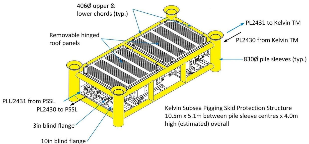
**Figure 2.3.2: Perspective of the Kelvin/Murdoch Subsea Pigging Skid protection structure**
