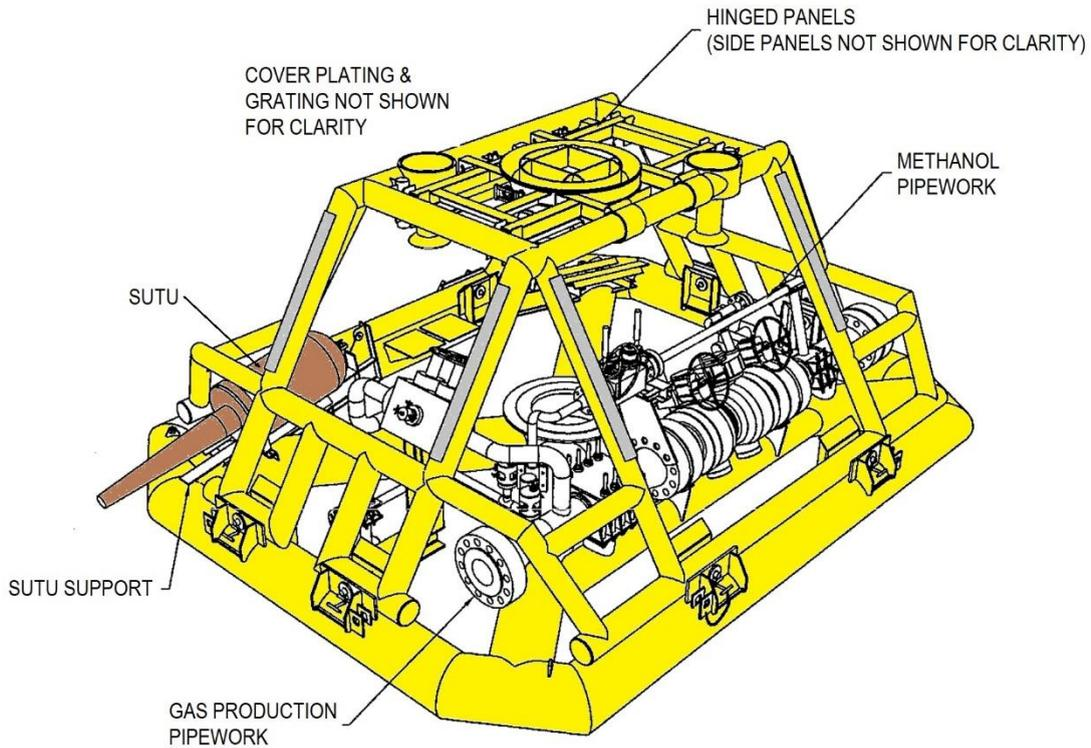
**Figure 2.2.2: Perspective of Hawksley EM subsea installation**
