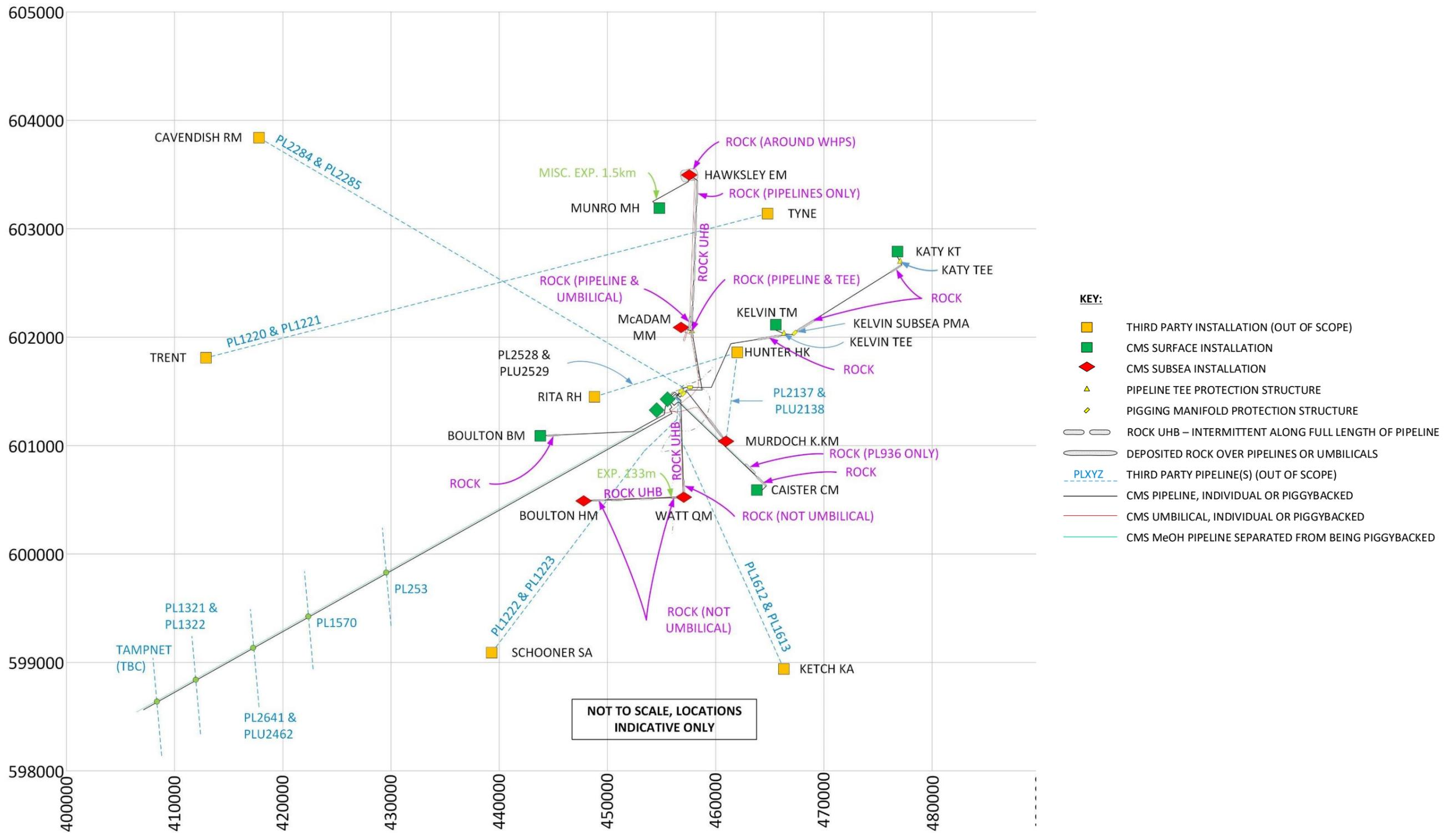
Figure A3.1.1: Schematic of deposited rock outside Murdoch 500m zone
