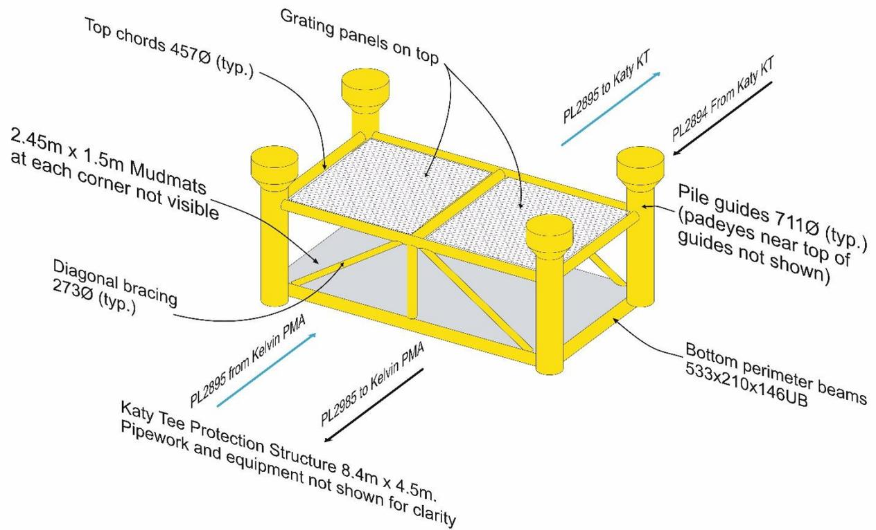
**Figure 2.3.1: Perspective of the Katy Tee protection structure**
