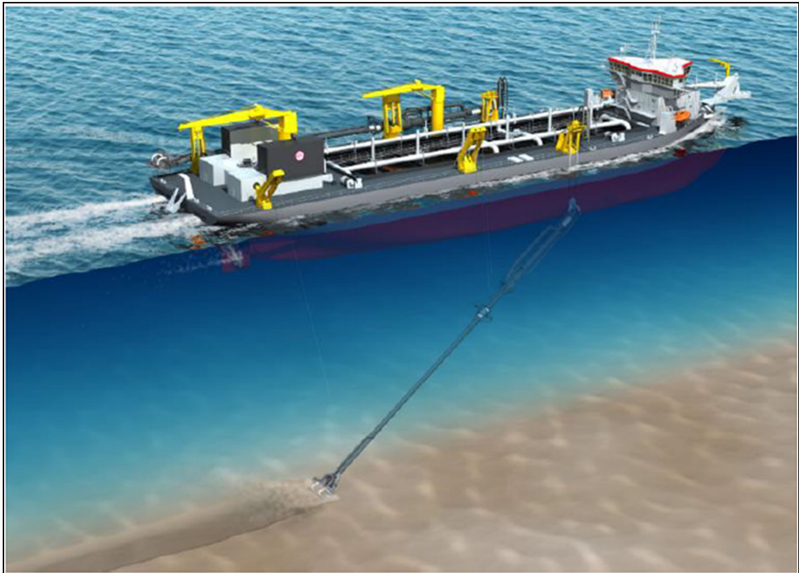
Figure 2-9 Trailing suction hopper dredger
