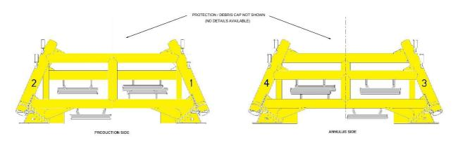
Figure 2.2.5: Elevation on WHPS for well P1 & W1 (protection cover not shown)
