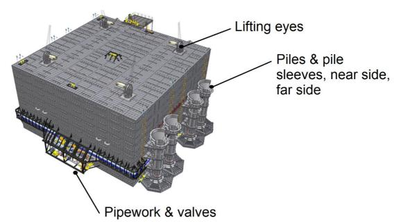
Figure 2.2.1: SOST 3D Schematic
