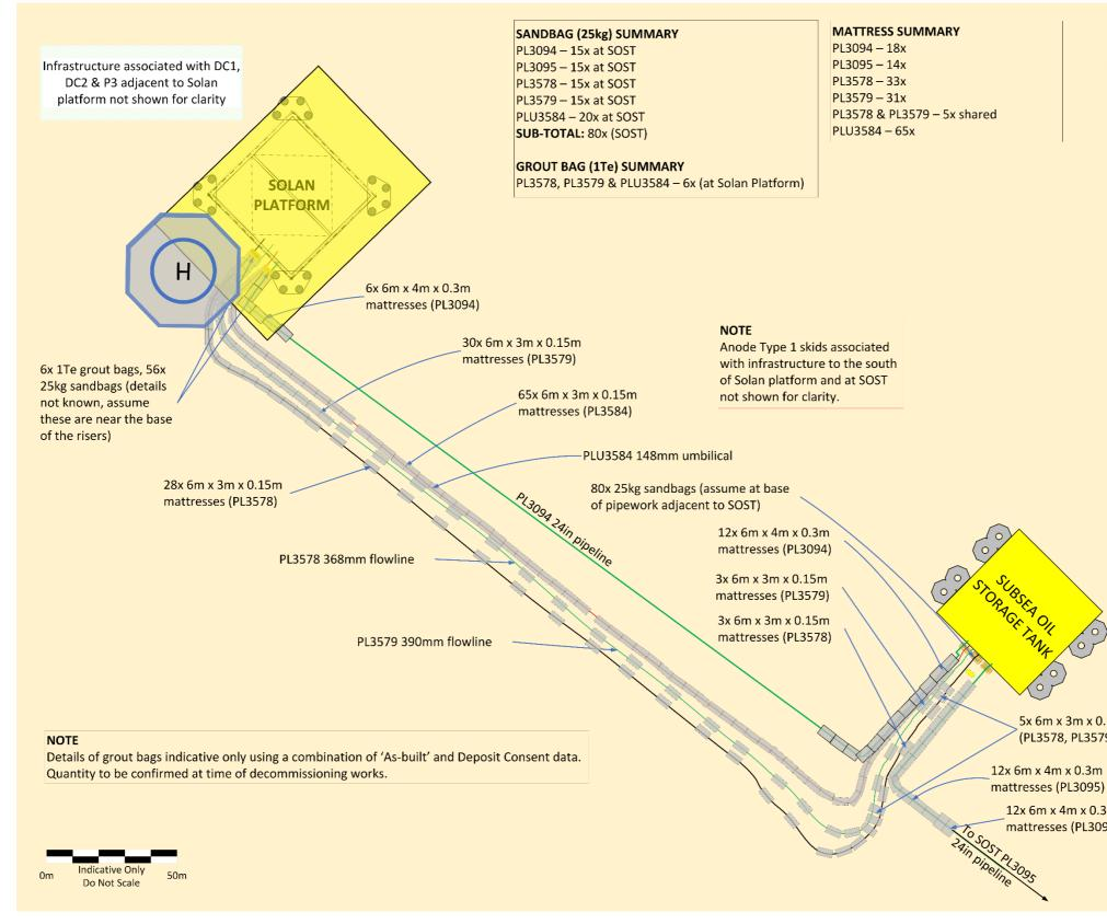
Figure 6.6.3: Solan platform and SOST infrastructure schematic
