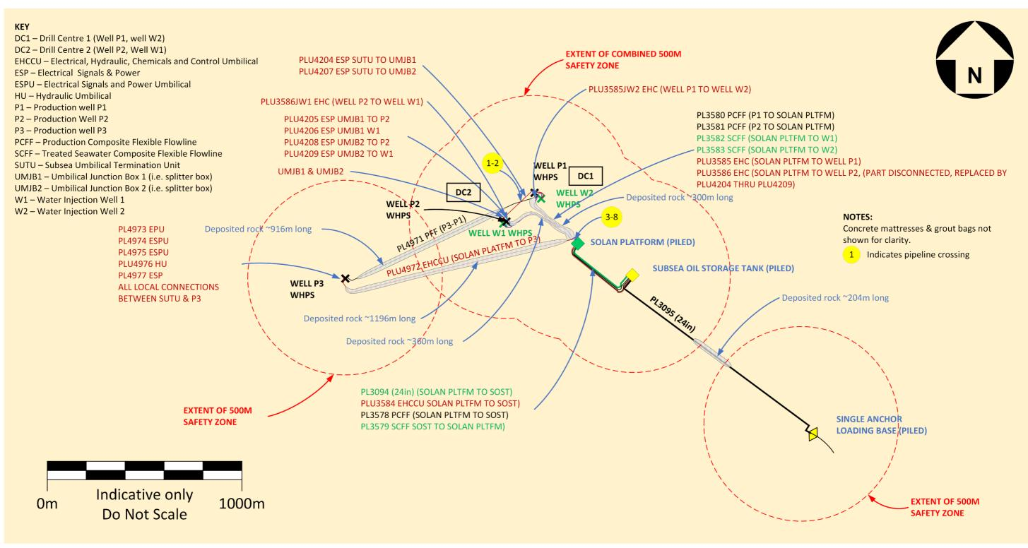
*Figure 6.6.1: Solan field infrastructure overview schematic*
