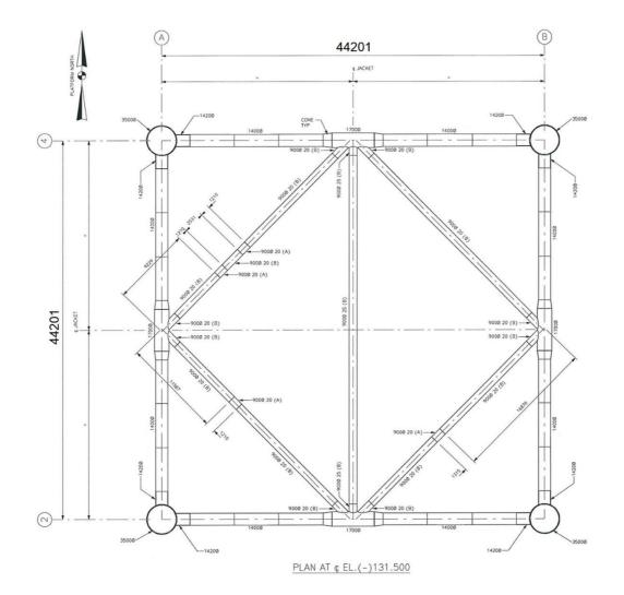
Figure 3.2.10: Solan jacket bracing plan at EL. -131.500
