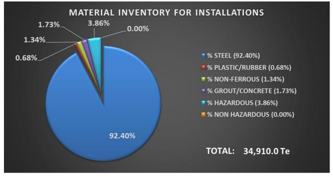
Figure 2.7.1: Material inventory for Solan installations<sup>3</sup>
