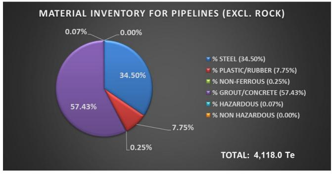
Figure 2.7.2: Material inventory for Solan pipelines<sup>3,4</sup>
