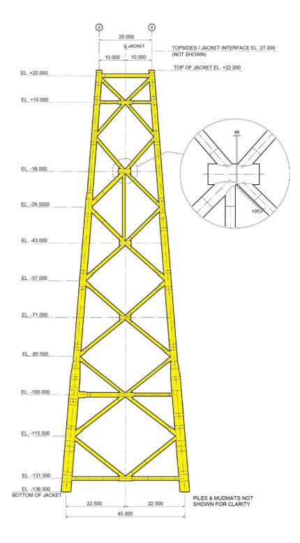
Figure 3.2.3: Solan jacket elevation on row 'A' (rows 'B', '2' & '4' similar)
