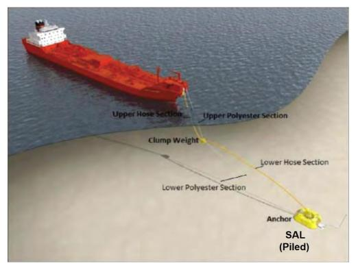
Figure 2.5.1: SAL system schematic
