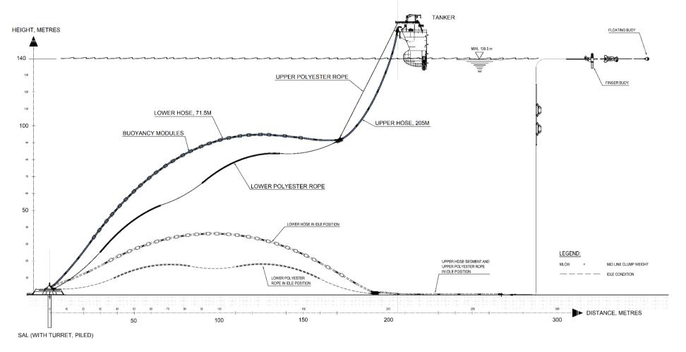
Figure 2.5.4: SAL hose pickup system
