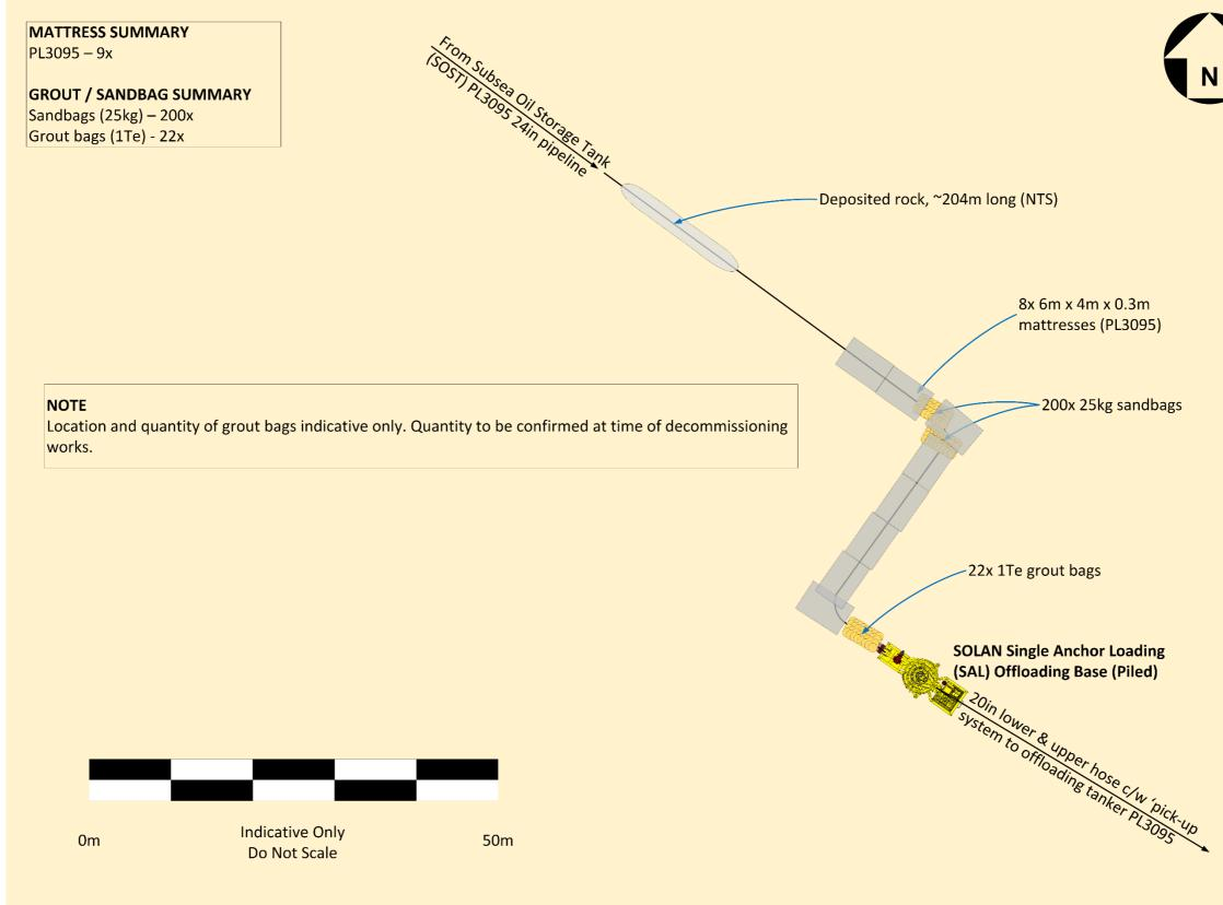
Figure 6.6.4: SAL approach schematic
