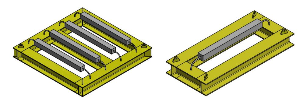
Figure 2.5.5: Anode skid type I (L) and type II (R)
