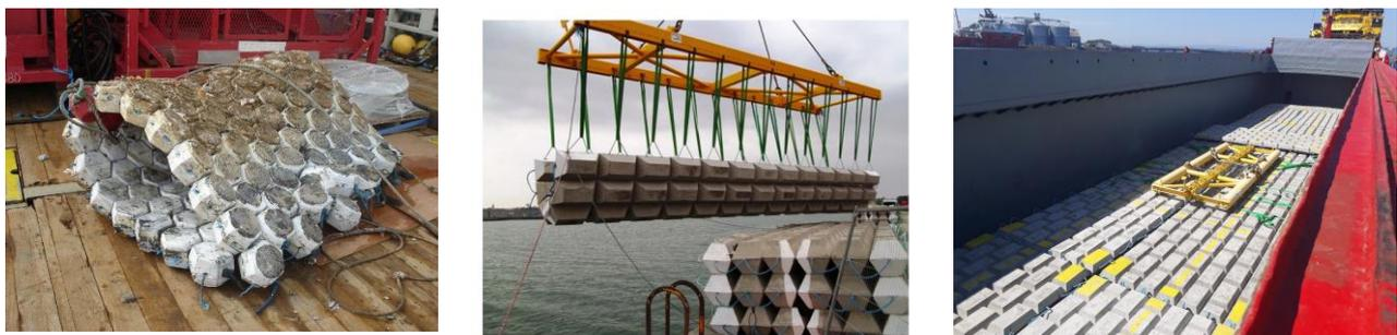
**Figure 2.4.7: Linklok, Fleximat and Biflex mattresses respectively (indicative only)**
