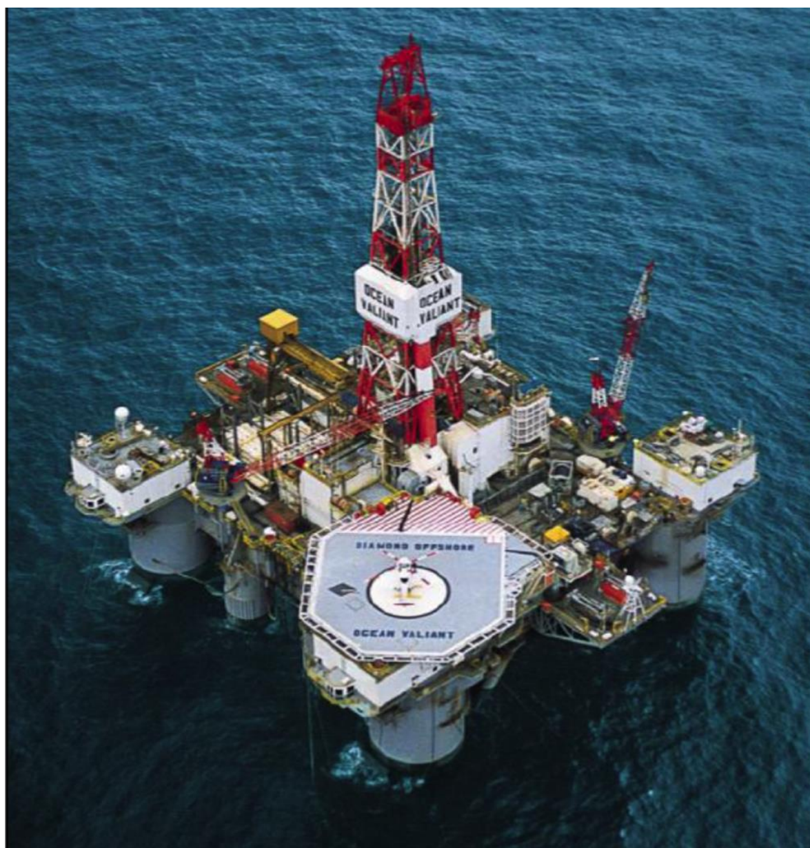
Figure 5.3: Photograph of a typical anchored semi-submersible drilling rig (the Ocean Valiant )
