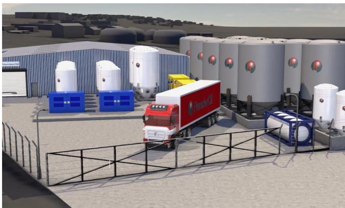
Figure 5.14: Schematic of the liquid mud plant to support exploration drilling campaigns
