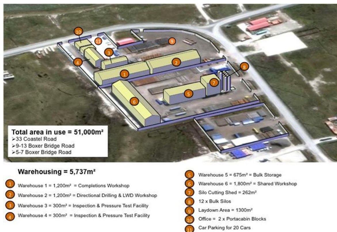
Figure 5.13: Schematic of the supply base developed to support exploration drilling campaigns
