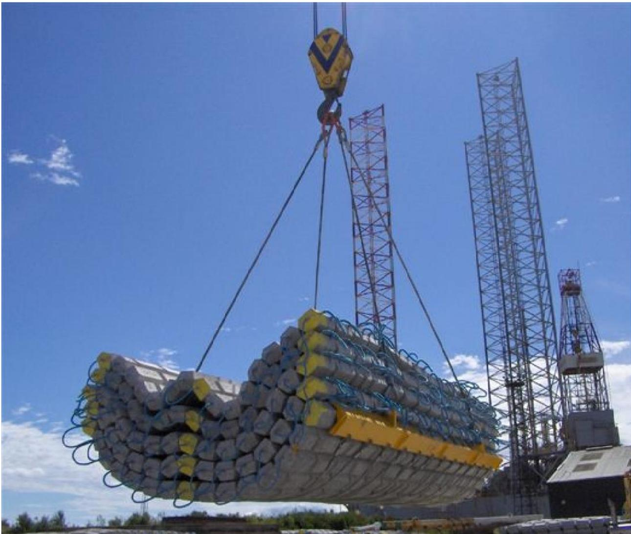
*Figure 5.4.2: Speedloader lifting frame<sup>21</sup>*
