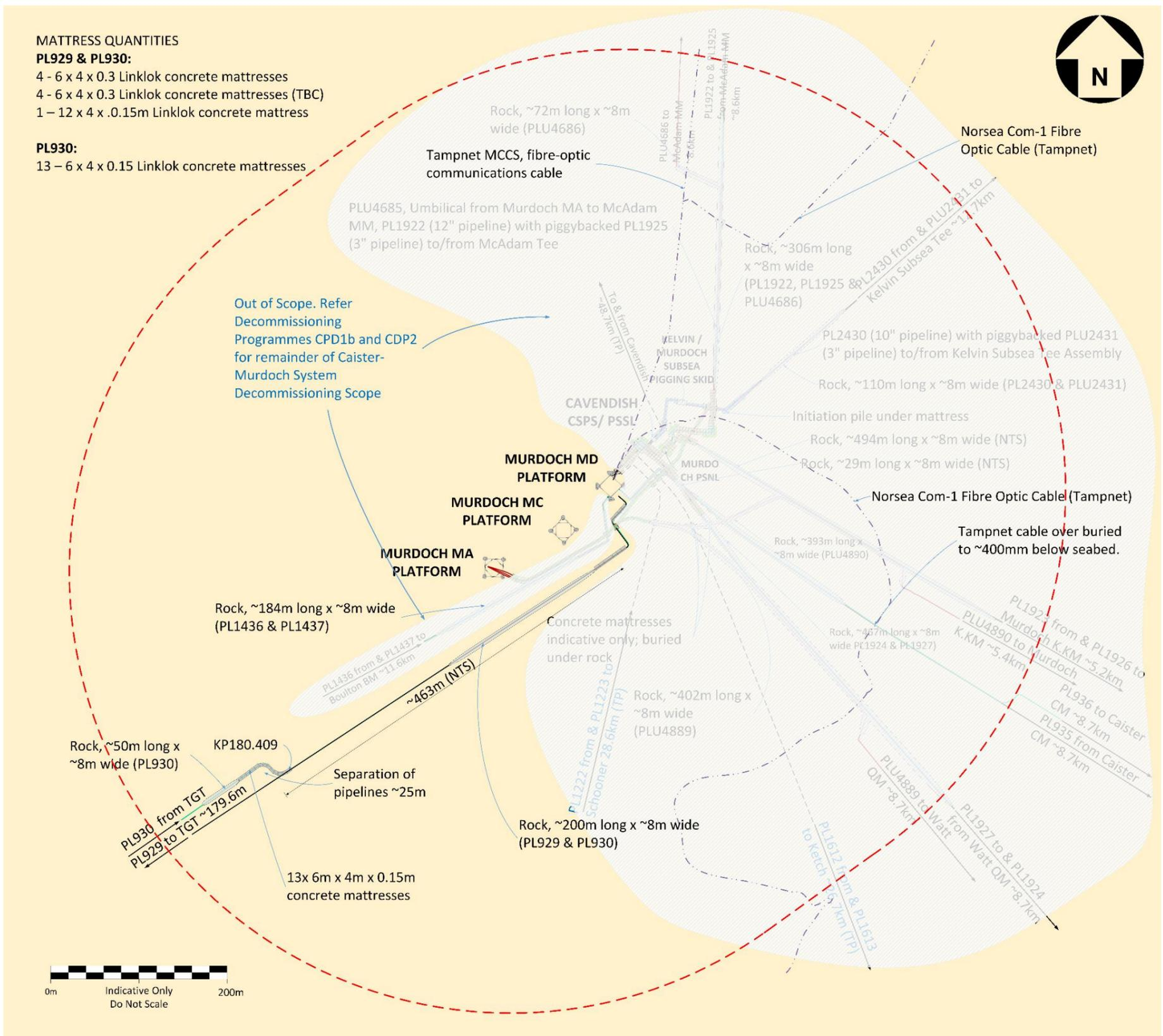
Figure 2.2.2: Murdoch installation 500m zone<sup>1</sup>
