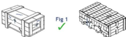
Crates with an open framework design as shown in Fig2, are not suitable for lifting by crane and should therefore not be shipped offshore
