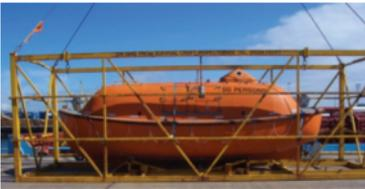
A yellow lifeboat is mounted on a yellow metal transportation frame. The frame is a rectangular structure with diagonal bracing, designed to hold the lifeboat securely during transport.                                                         |
