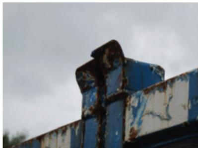
2. The equipment/materials packed within a CCU in a manner which creates the potential for the lifting set to snag on it.
