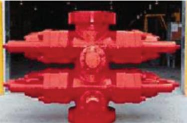
A large, complex, red-painted metal frame for a Blow Out Preventer (BOP). It has a central vertical section with several horizontal arms extending outwards, all supported by a sturdy base.                                                      |
